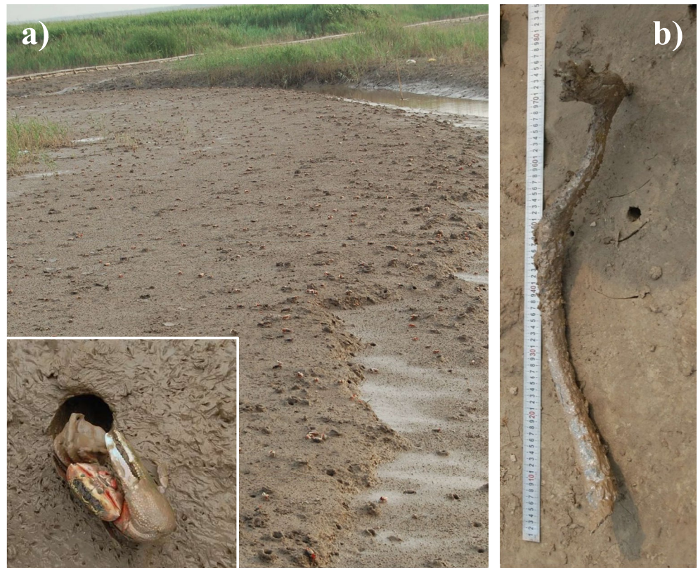
Figure 6. (a) Macropores (crab burrows) distributed in marsh soils. An Uca arcuata crab is shown at the lower left corner. (b) Morphology of a crab burrow taken using polyester resin casting (Chongming Dongtan wetland, China; images captured by P. Xin on 11 July 2007).
